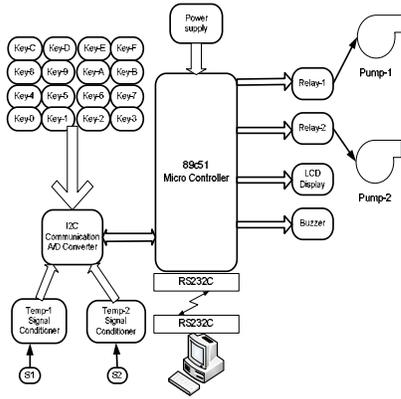
Fig 3.1 TMCNRS Hardware Integration diagram
