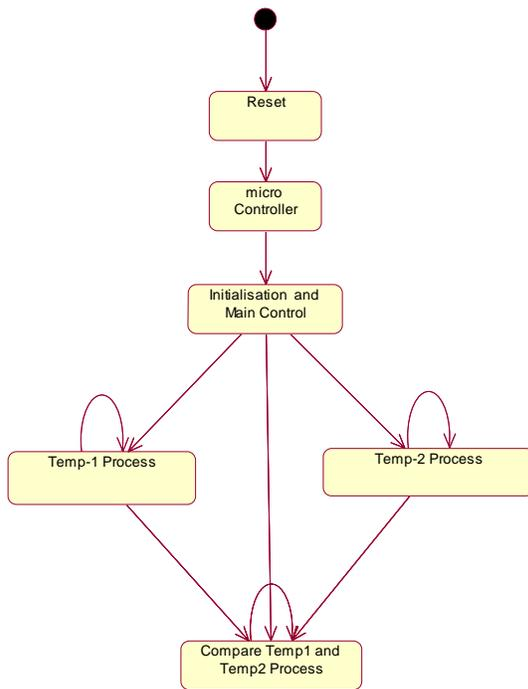
**Figure 4.11 Top Level state diagrams**
