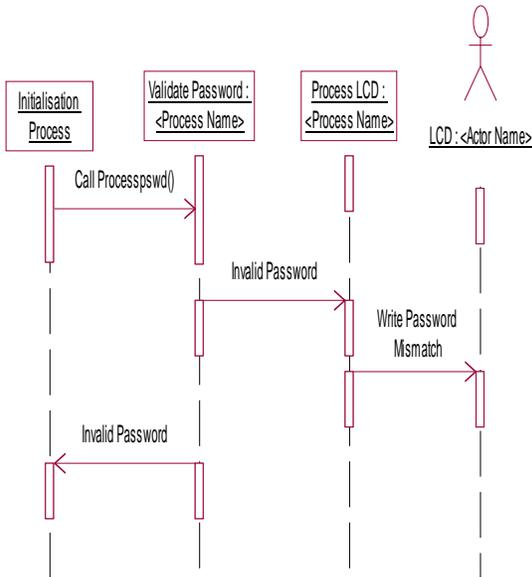
4.7 Processing flow for validating the password
