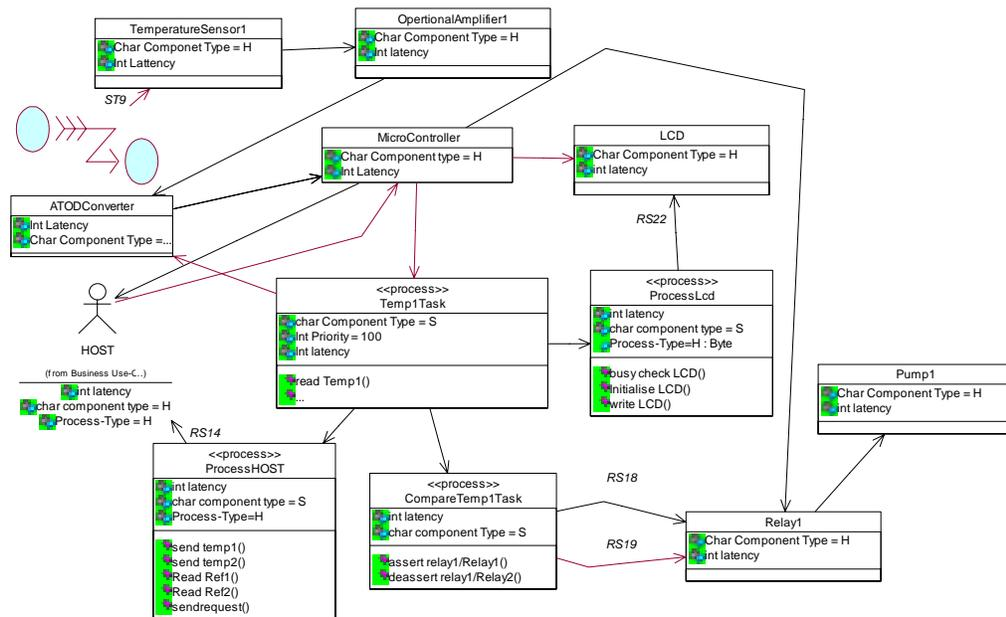
Fig 4.2 Class Diagram for processing Temperature-1
