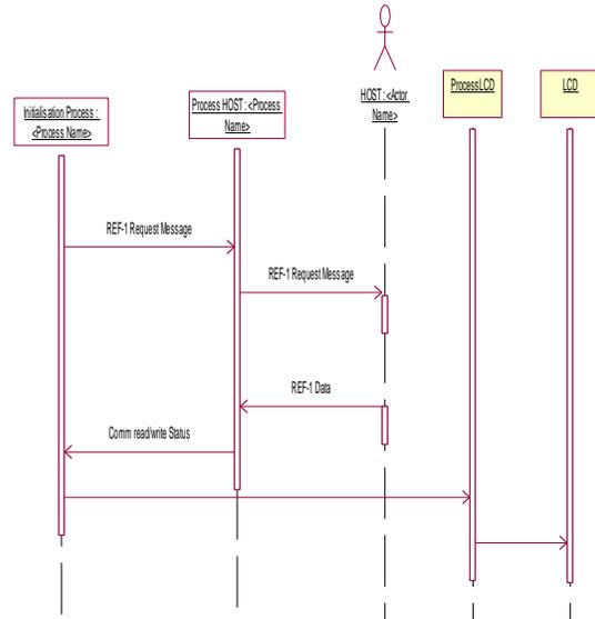
Figure 4.9 Sequence Flow for reading Reference Temperature -1
