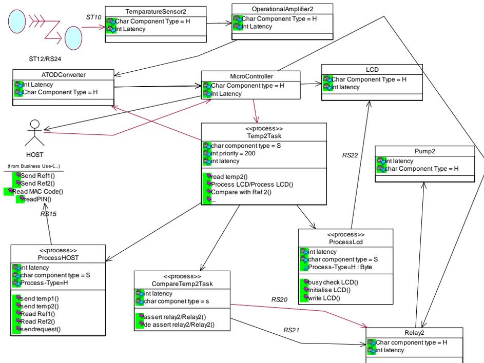
Fig 4.3 Class Diagram for processing Temperature-2
