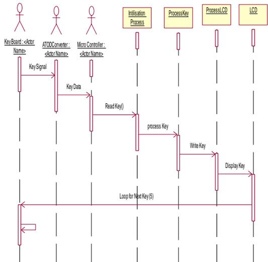
4.6 Processing flow for capturing keys related to entered password
