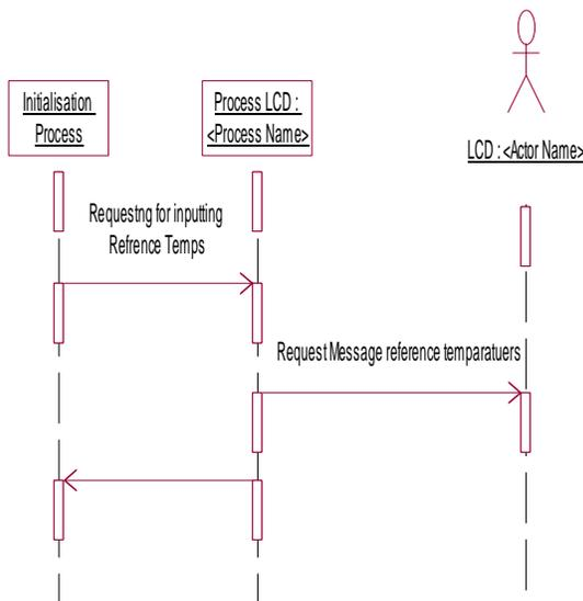
Figure 4.8 Sequence flow for processing the request for inputting the reference Temperatures
